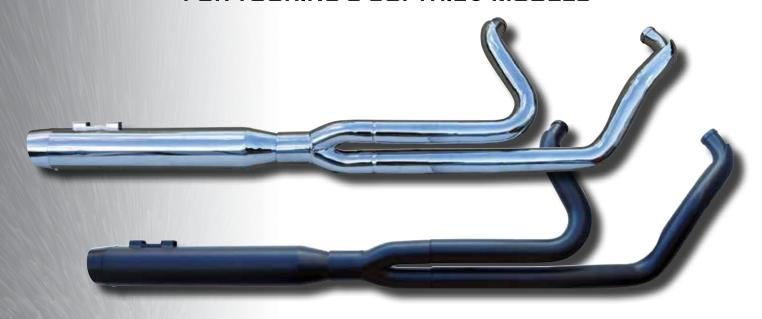
These Ultima® Touring 2 into 1 exhausts have it all, good looks, competition inspired performance, and an excellent exhaust tone. Baffles, O2 Sensor plugs and full length heat shields included and installed.
