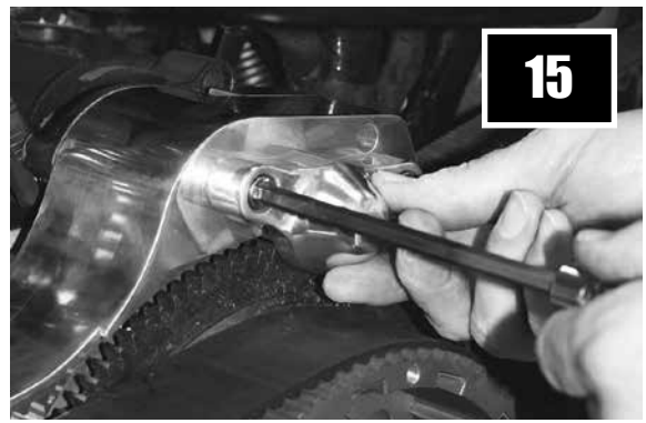
15. Install the starter jackshaft cover using blue thread locker on the bolts.
