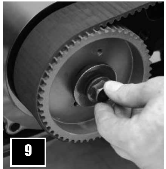
9. Install & torque the OEM compensator bolt to manufacturers specs. Always clean bolt thoroughly and apply red thread locker before installing.
