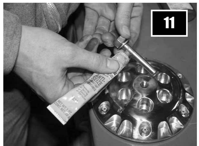
11. Install the clutch adjusting screw using a small amount of high temp grease or antisieze on the threads & on the clutch pushrod end.
