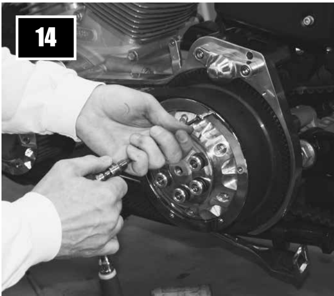
14. Install the chromed belt guide using blue thread locker on the bolts.
